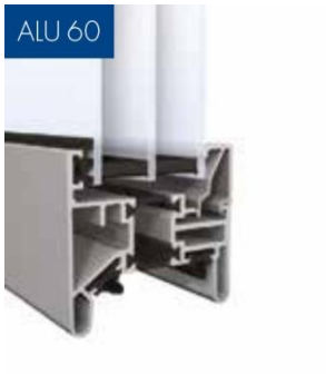
Panorama door 60 mm Triple Plexiglas Optical 40 mm (4-14,75-2,5-14,75-4 mm) U-value of the Panoramic door 60: 4,000 x 4,000 mm: 2.45 W/m 2 K
