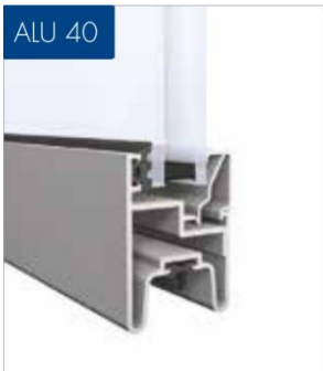
Panorama door 40 mm Double Plexiglas Optical 20 mm (4-12-4 mm) U-value of the Panorama door 40: 4,000 x 4,000 mm: 4.35 W/m 2 K
